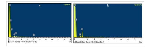
Fig. 3: EDX of MCC obtained from Apricot stone Shells [a] S5 and [b] S6.
