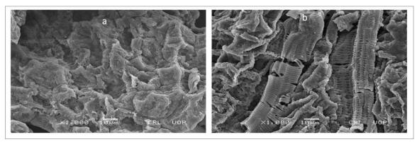
Fig. 6: SEM images of MCC obtained from Apricot stone shells [a] S4 and [b] S6.
