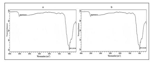
Fig. 8: FTIR spectrum of MCC obtained from Almond shells [a] S3 and [b] S4.
