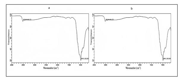
Fig. 9: FTIR spectrum of MCC obtained from Apricot stone shells [a] S5 and [b] S6.
